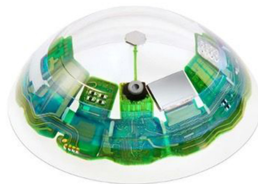
Figure 1 The prototype Mojo Vision smart contact lens with a 14 000 pixels per inch micro-LED display, the world's smallest at just 0.5 mm in diameter, and densest with a pixel-pitch of just 1.8 µm, 5G ultra-low latency radio to stream AR content, continuous eye tracking via custom-configured accelerometers, gyroscopes and magnetometers, medical-grade in-lens batteries and eye-controlled user interface. 2 AR, augmented reality; LED, light-emitting diode.
