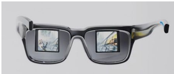
Figure 2 The vision enhancement technology by Innovega is made of display glasses and a smart lens that picks up the images and media from the eyewear display and projects it directly on the retina. Outer filters allow one to see the natural world simultaneously while preventing cross-talk between light paths. 3
